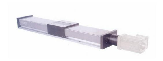
The COVERED LINEAR TABLES, are translation units almost identical to the Standard Linear Tables. The main difference lies in the fact that these are equipped with a metal cover that protects the most sensitive components such as: the guides, the screws, the nuts, the linear bearings, etc.
