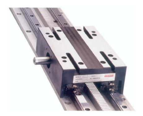
NIASA's GLC rack-pinion linear guides are translation units with no travel limitation. Their simple design and great robustness transform them into very useful elements for mechanisation. They are equipped with precision ball guides designed to support heavy loads, extremely high rigidity, maximum precision and very low noise levels.
